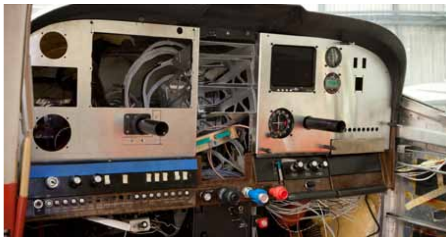
Line drawing (top) shows the airplane's instrument cutouts, and bottom photo shows the panel's progress as of early January. Advantage's Mark Krueger (above left) traces an old instrument panel—not ours—using a digitizer that recreates the panel's exact dimensions. After this step, the new panel is laid out with AutoCAD software, cut by a CNC machine, powder coated, and laser engraved. Advantage's shop (top right) has a showroom of avionics suites. Garmin's G500 (above right) is the heart of the panel to be.
